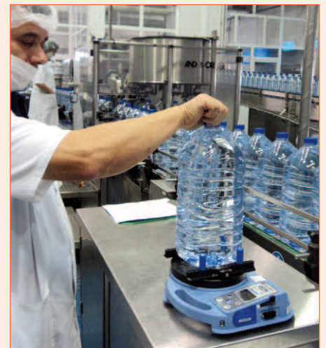
PET bottle cap test on a Tornado digital torque tester
